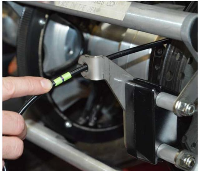
7. Install cable clevis on caliper actuator lever.
