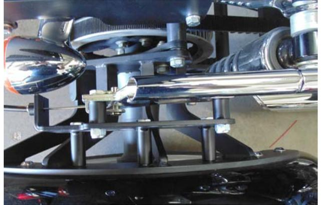
6. Mark the length of the housing. Cable needs to be longer than the housing. **Do not cut the cable now. Remove housing from the cable.** Use an abrasive cut off wheel to cut the housing. **Do not Smash the housing**
