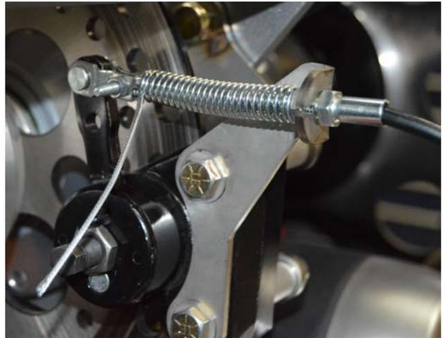
12. Use the cable adjuster to take up the slack in the housing. Lift the parking brake handle to test the brake. Adjust until the parking brake holds. Release the handle and make sure the caliper releases.
