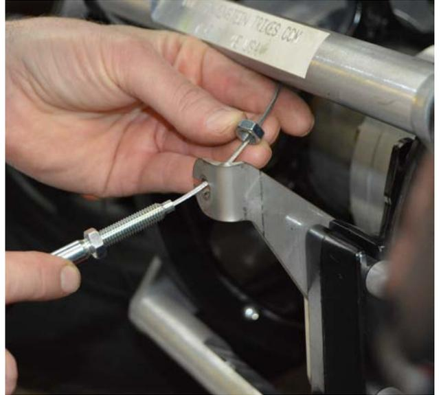
9. Install spring over cable, thread cable through cable clevis. Make sure that the cable adjuster is bottomed out. (no threads showing on the back side of the bracket as shown in picture) Hold lever forward with your thumb, pull cable snug around clevis. Wrap electrical tape around cable where you want to cut the cable. Leave enough extra cable so you can get a good grip.
