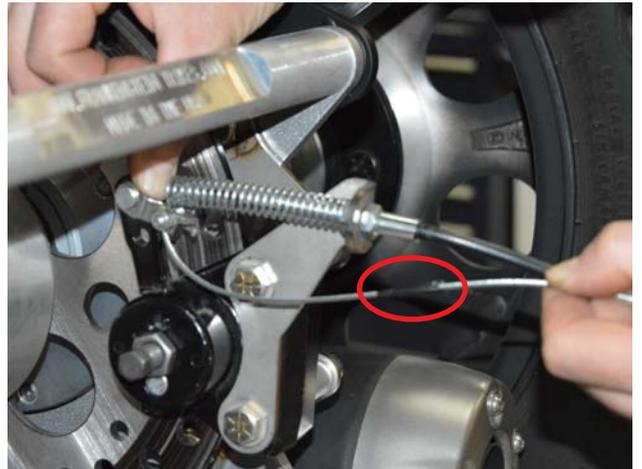
10. Pull cable out of clevis, remove spring and adjuster. Cut cable with abrasive cut off wheel in the center of the electrical tape so the cable won't fray.
